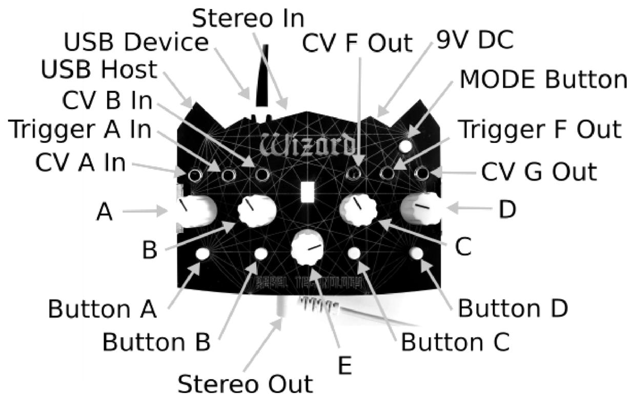
To change the output volume of the device, hold down the MODE button (top right corner) and turn the D knob (right side) to adjust.
